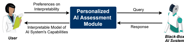
Figure 1: The personalized AI assessment module uses the user’s preferred vocabulary, queries the AI system, and delivers an interpretable model of the AI system’s capabilities.
