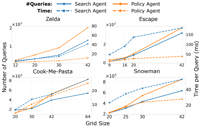
Figure 3: Performance comparison of search-based agents and policy-based agents in terms of the number of queries asked and time taken per query when increasing the grid size (number of cells in the grid) in the four GVGA domains.
